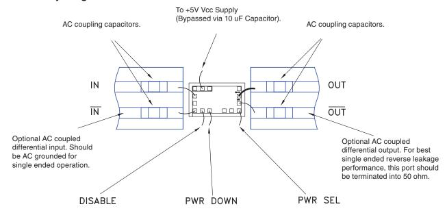
This port should be grounded for normal operation. Applying +5V to this port will disable the input buffer amplifier.
